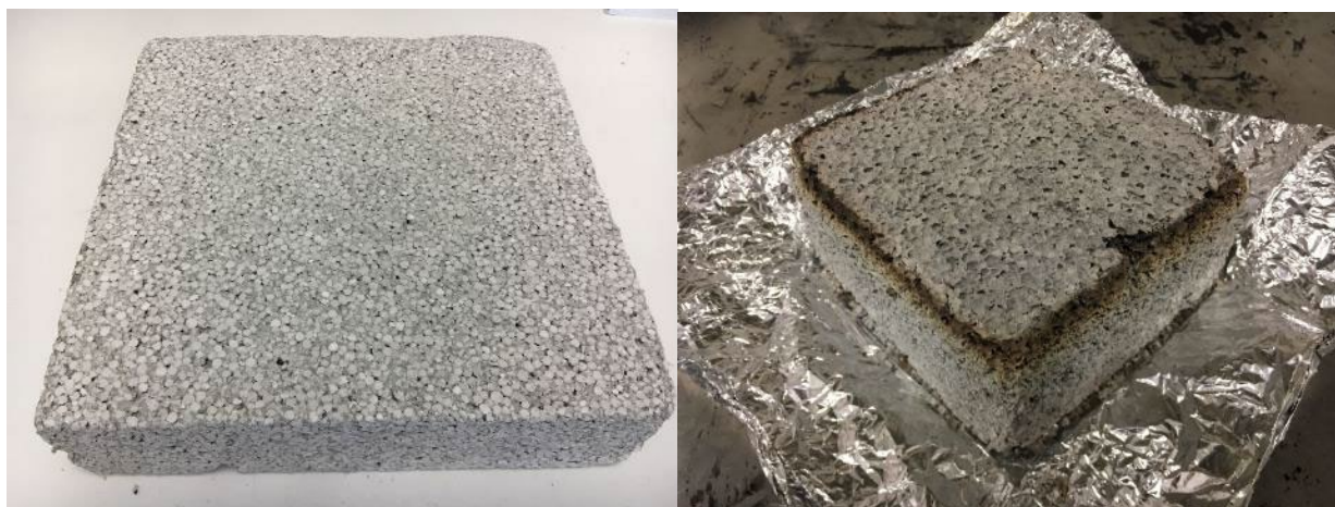
Figure 11. Conpolcrete prior to cone calorimeter test (left) and after cone calorimeter test (right) – All photos by CSIRO
