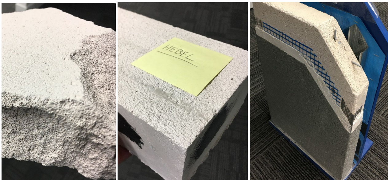
Figure 1. typical AAC structure (left), Hebel block (centre), Typical AAC EIFS installation (right), all photos by CSIRO.
