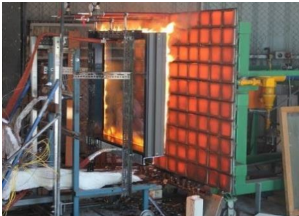
Figure 19. CSIRO pilot scale AS 1530.8.1 test (left), BAL radiant heat test profiles (right)
