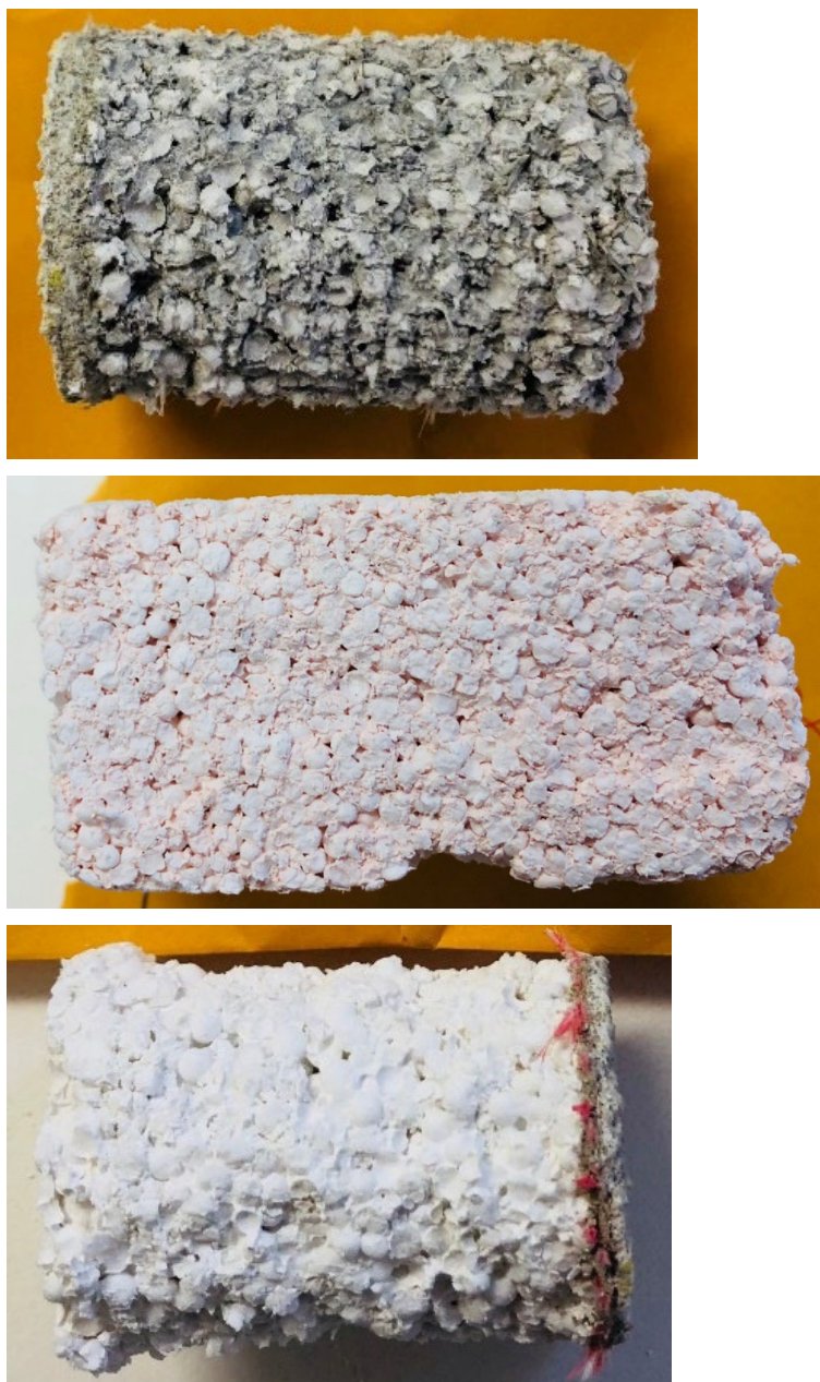
Figure 8. Examples of State-wide Cladding Audit Conpolcrete® samples provided by VBA from existing buildings. Grey Conpolcrete® (top), Pink Conpolcrete® (middle), White Conpolcrete® (bottom)
