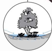
Garden beds with deep friable soils can help to slow, filter and collect water
