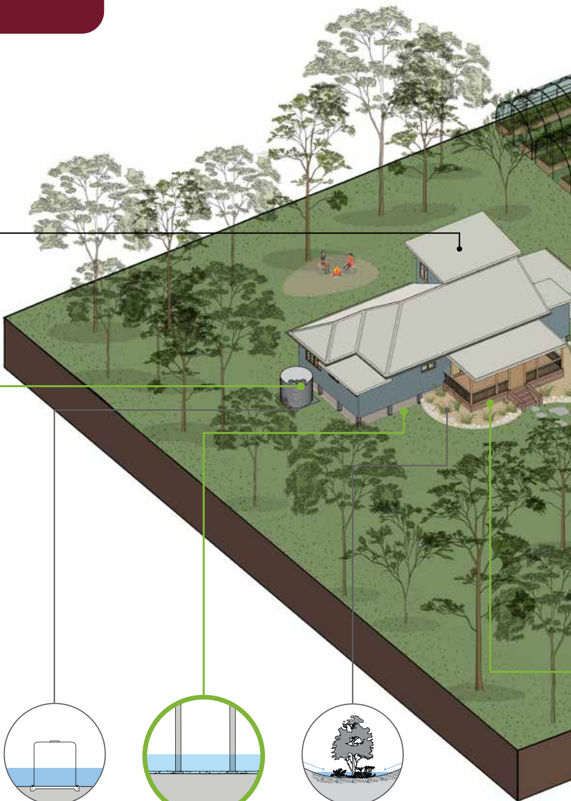
Install water tanks to collect rainwater. Ensure unit is secured to ground.
