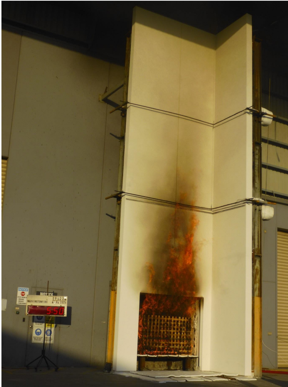
Figure 34 The external wall system during the test – 5 minutes 50 seconds after crib ignition
