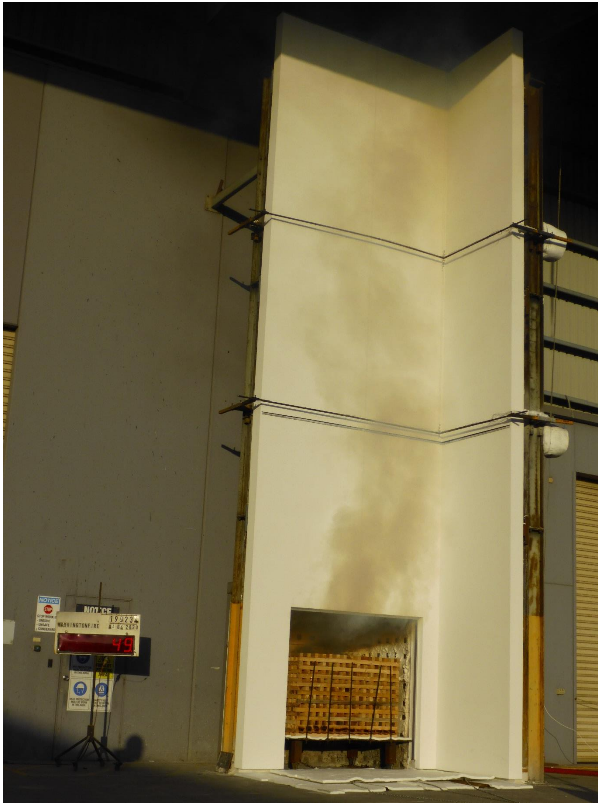
Figure 32 The external wall system during the test – 49 seconds after crib ignition
