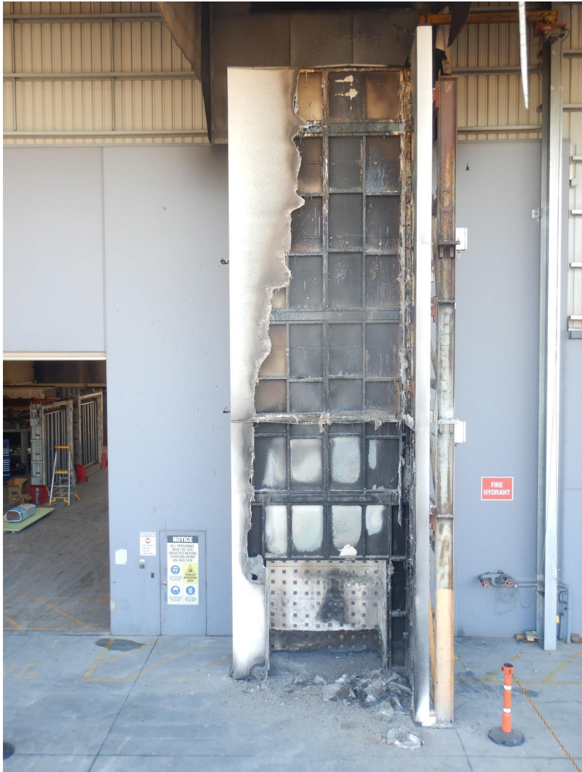
Figure 45 The post-test external wall system with the severely heat damaged render removed – main wall
