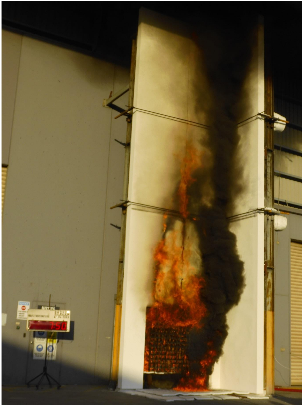
Figure 36 The external wall system during the test – 7 minutes 50 seconds after crib ignition
