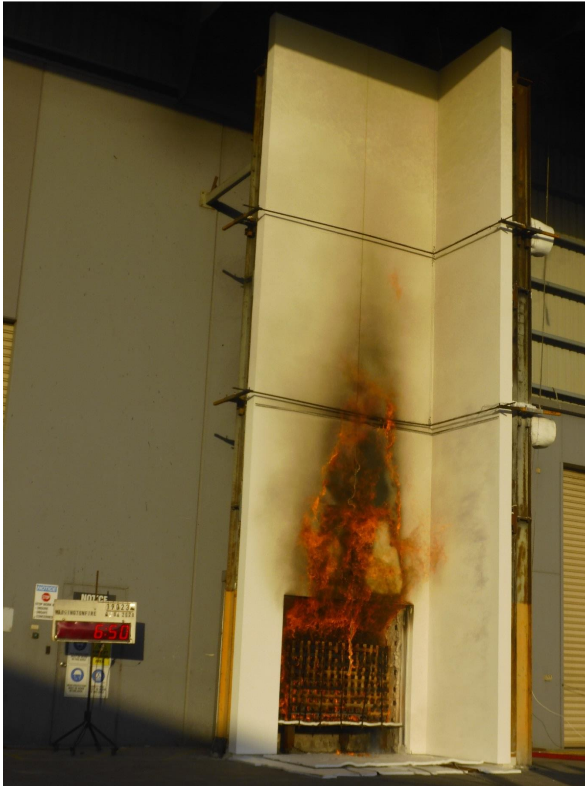
Figure 35 The external wall system during the test – 6 minutes 50 seconds after crib ignition
