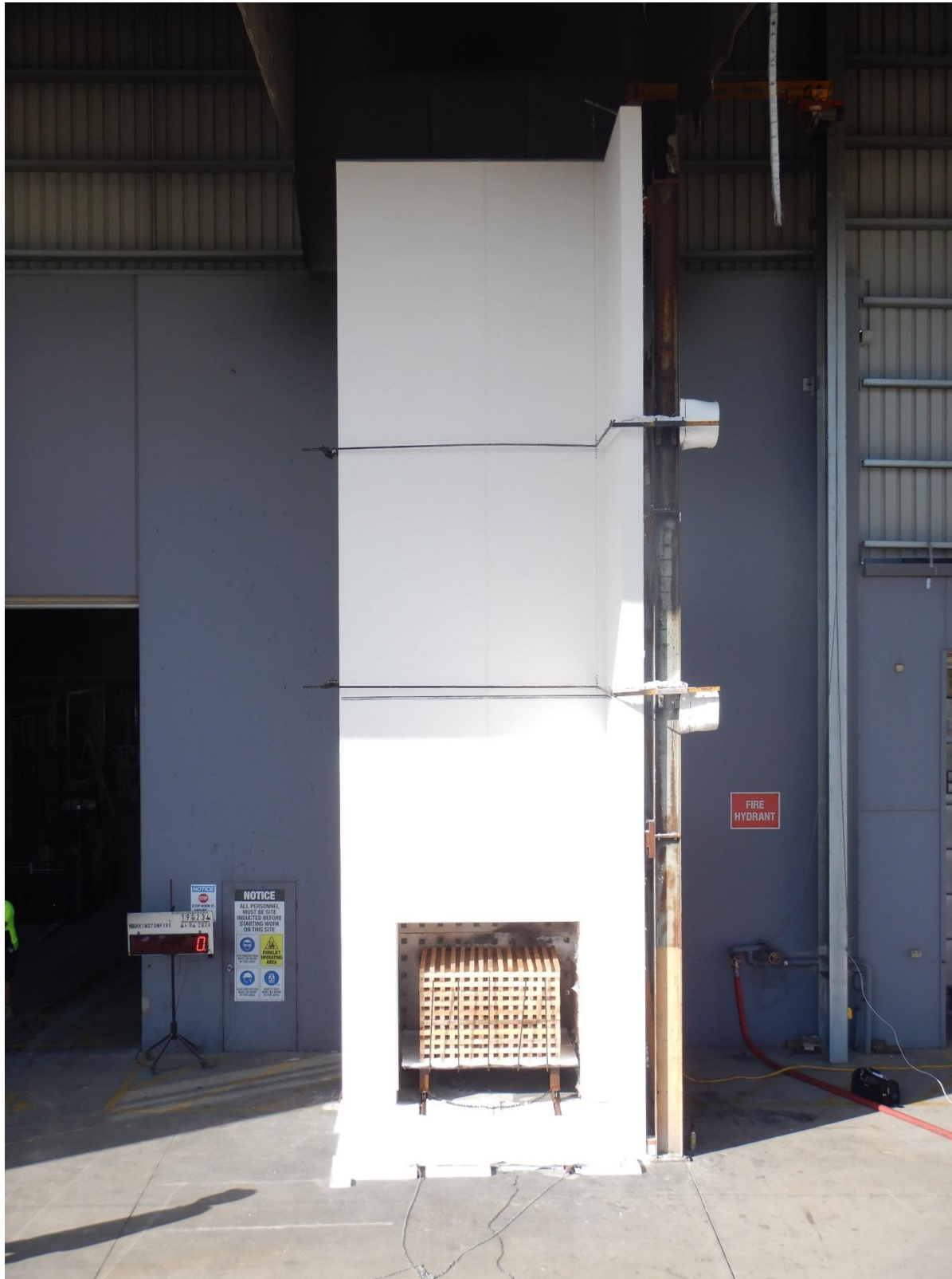
Figure 28 The complete external cladding system before the start of the test – main wall
