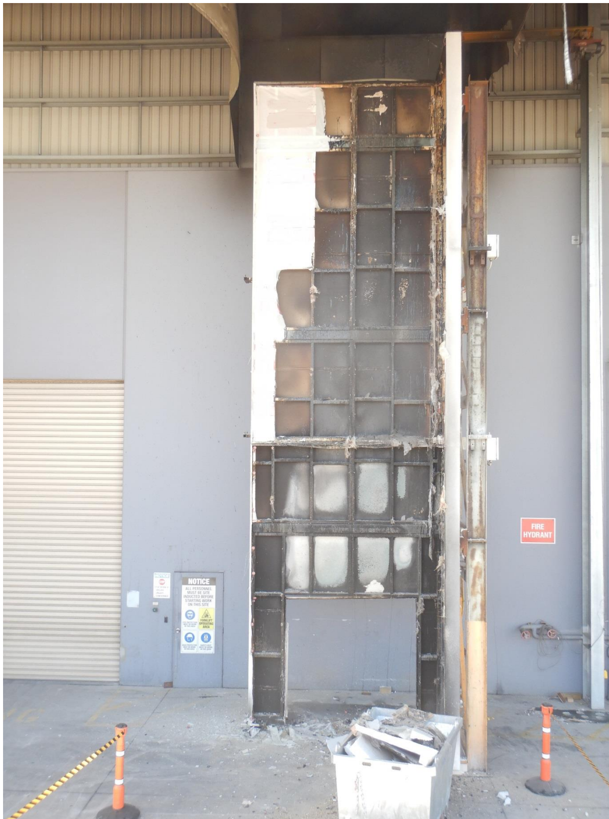
Figure 49 The post-test external wall system with all EPS panels removed – main wall.
