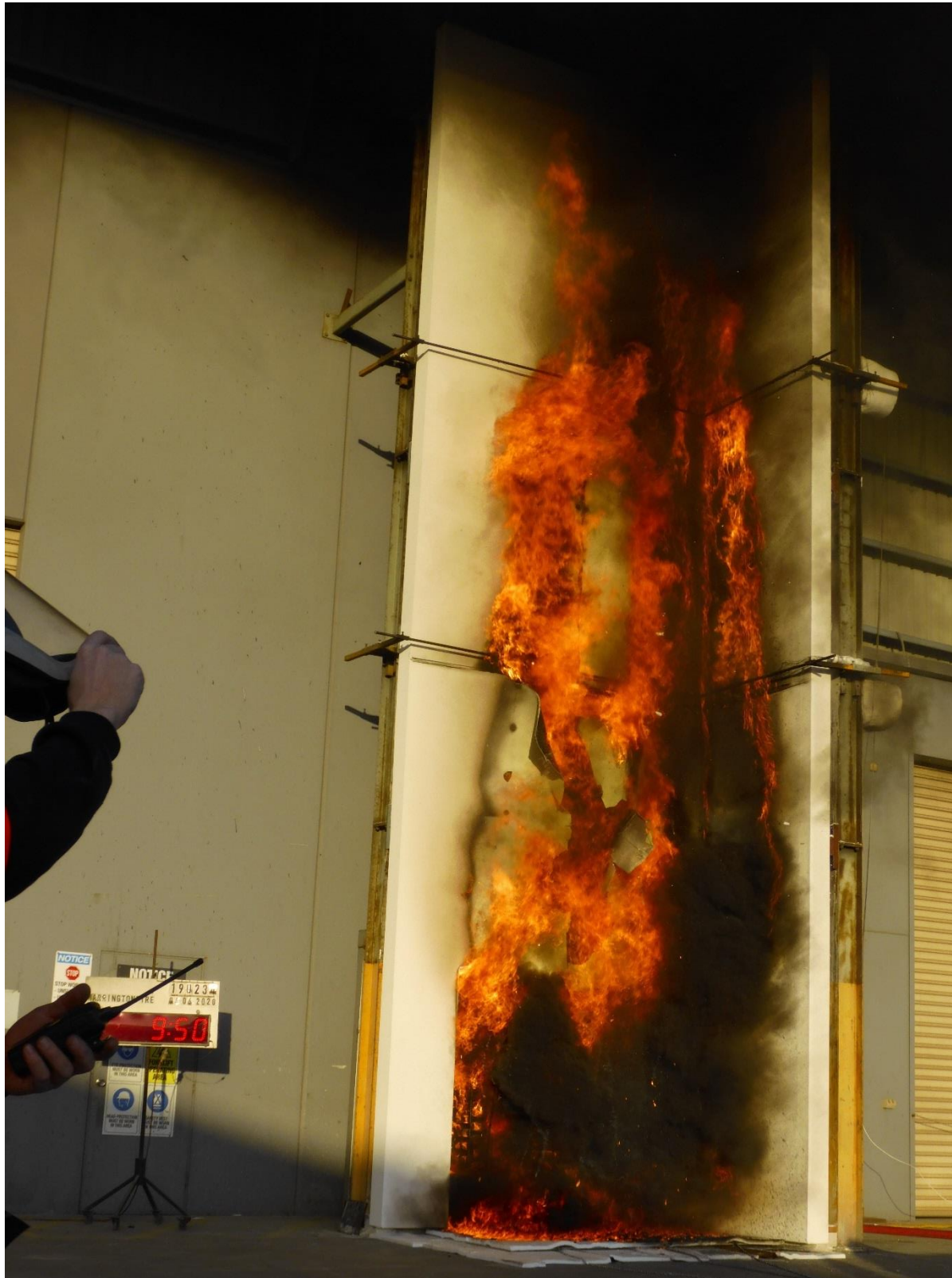
Figure 38 The external wall system during the test – 9 minutes 50 seconds after crib ignition
