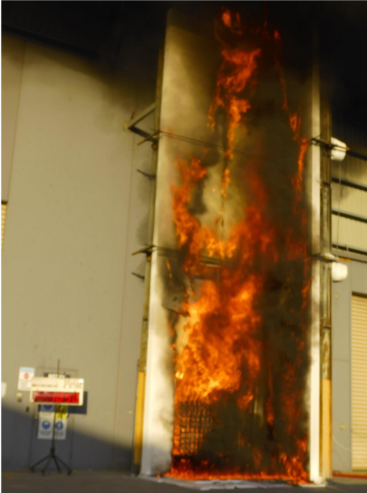
Figure 39 The external wall system during the test – 10 minutes 50 seconds after crib ignition
