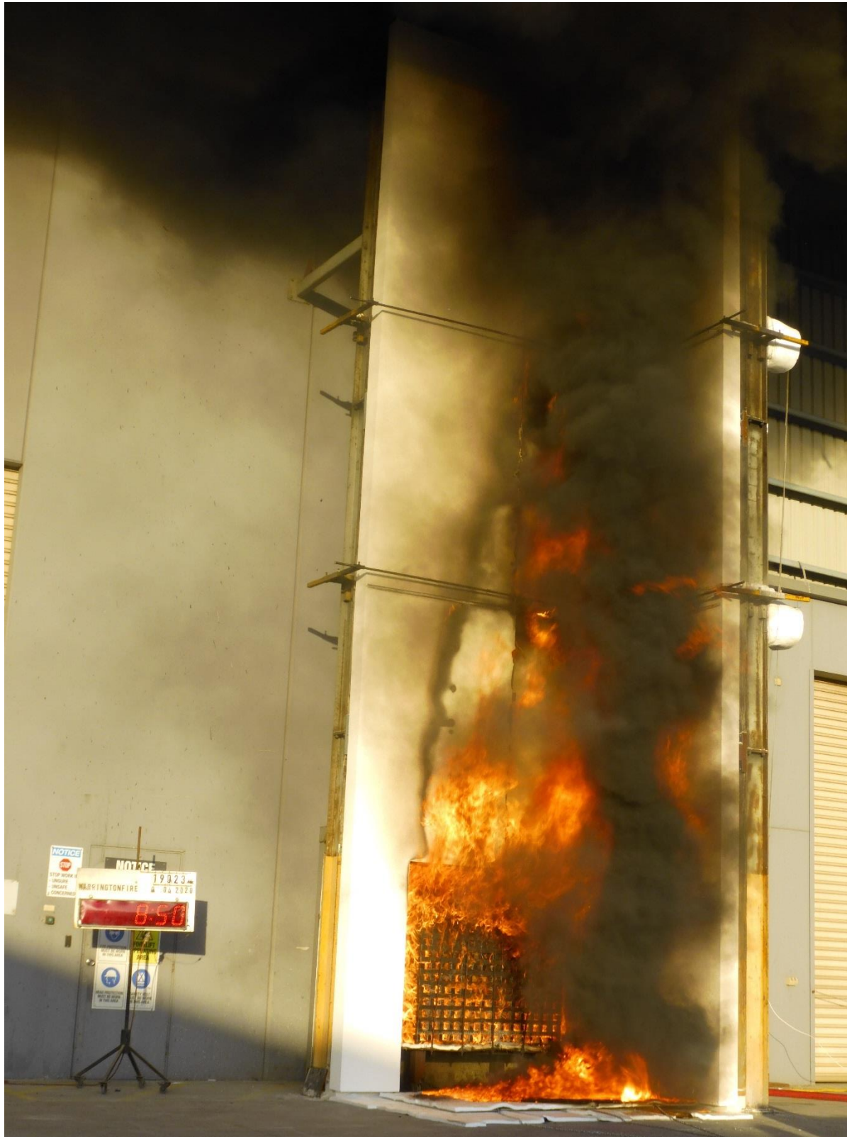
Figure 37 The external wall system during the test – 8 minutes 50 seconds after crib ignition
