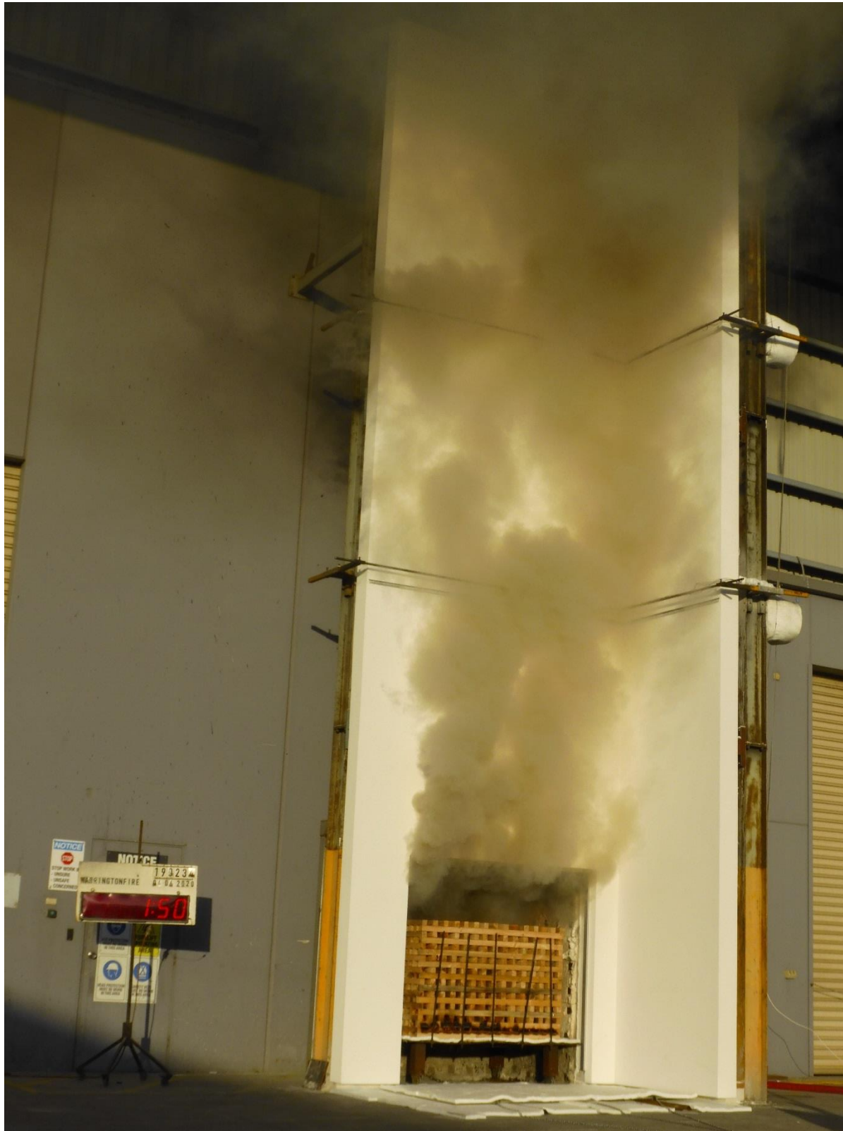
Figure 33 The external wall system during the test – 1 minute 50 seconds after crib ignition
