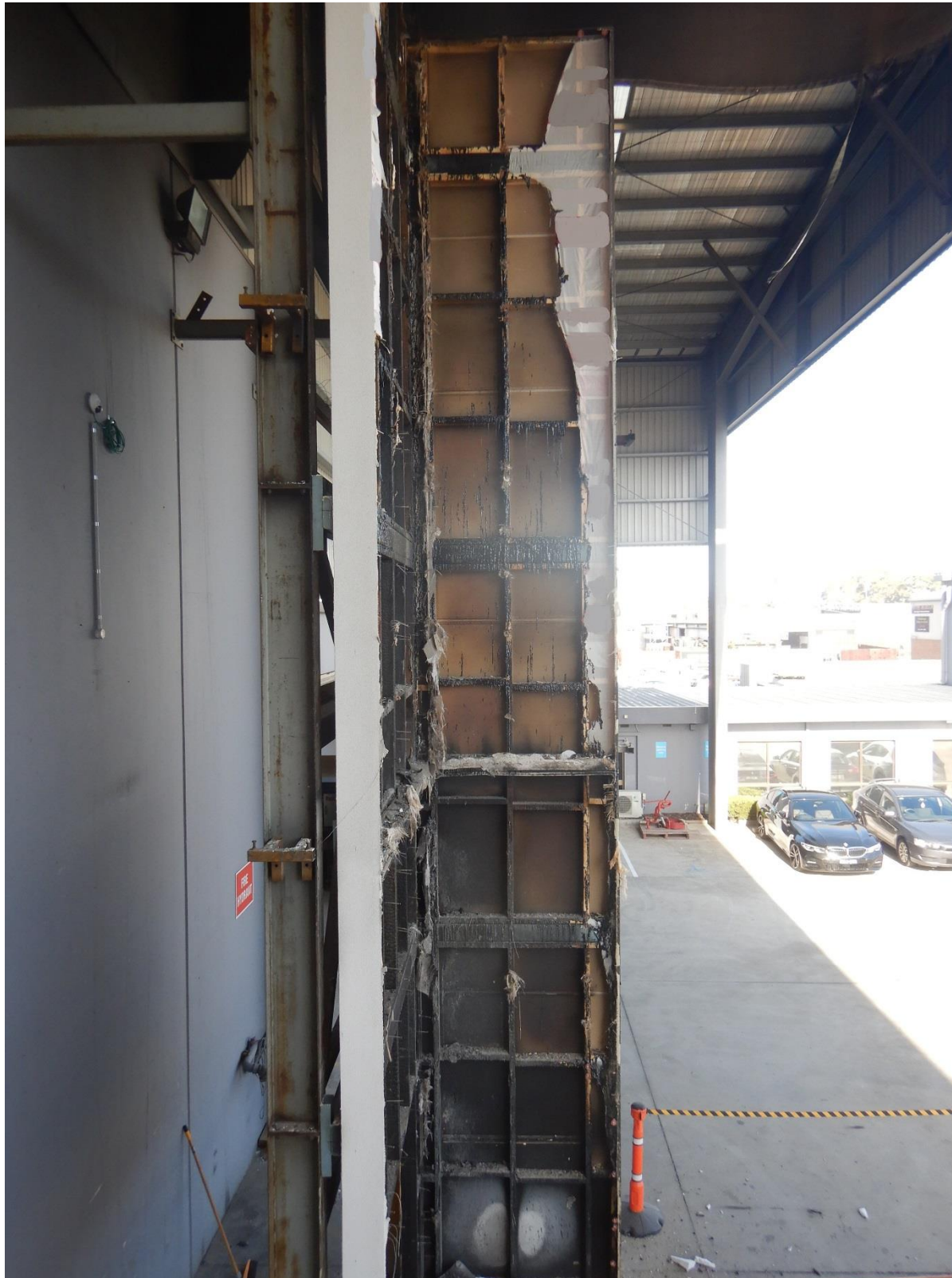
Figure 50 The post-test external wall system with all EPS panels removed – wing wall N.B. Image has been doctored to remove the branding from the sarking.
