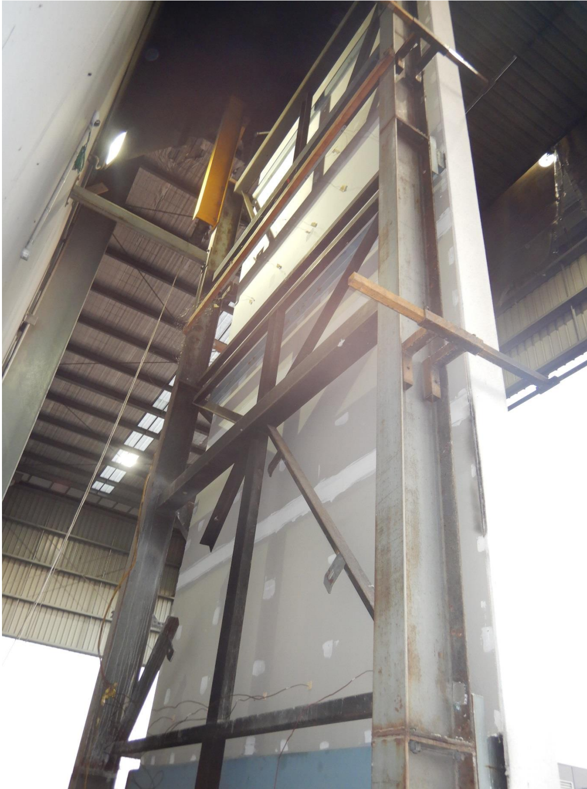
Figure 43 The unexposed side of the external wall system on completion of the test – main wall
