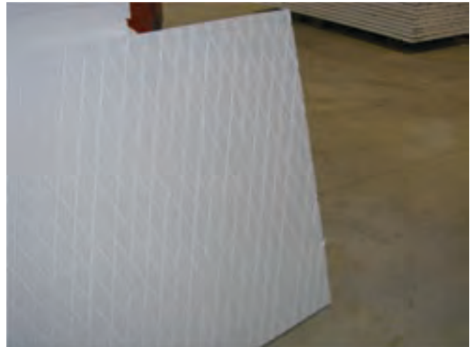
Photograph 5: “Groovy” - Cutting grooves into the continuous insulation to facilitate drainage also provides redistribution of moisture.
