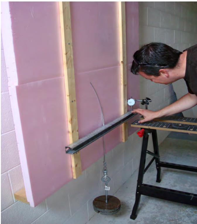
Photograph 5 – Deflection Testing - We have hung things off of foam sheathing to figure out deflection and moments. We have sucked on windows installed over continuous insulation to understand wind loading. We have blown on windows installed over continuous insulation to understand wind loading. Others have done this. Lots of others have done this. Even the foam industry has done this.
