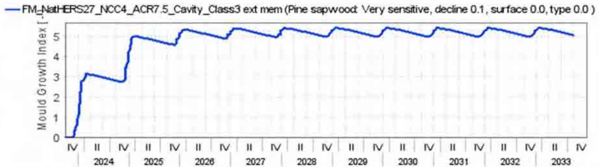
Figure 21: Flat Metal Cladding NatHERS CZ 27 - NCC CZ 4 South orientation ACR 7.5 With Cavity – Ext. Memb. Class 3 – 1398 – Mould growth within insulated timber frame
