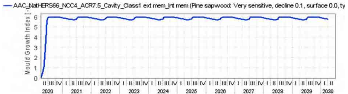
Figure 62 Autoclaved aerated concrete masonry NatHERS CZ 66 - NCC CZ 4 South orientation ACR 7.5 With Cavity – Ext. Memb. Class1 – 200000 with Int. Memb. Mould growth within insulated timber frame
