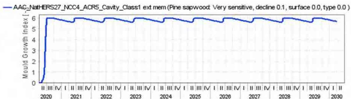
Figure 17: Autoclaved aerated concrete masonry NatHERS CZ 27 - NCC CZ 4 South orientation ACR 5 With Cavity – Ext. Memb. Class 1 – 200000 Mould growth within insulated timber frame
