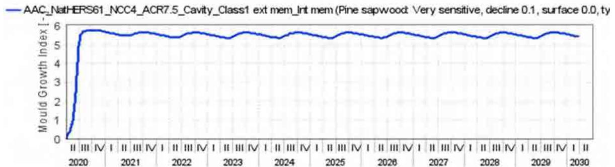
Figure 38 Autoclaved aerated concrete masonry NatHERS CZ 61 - NCC CZ 4 South orientation ACR 7.5 With Cavity – Ext. Memb. Class1 – 200000 with Int. Memb. Mould growth within insulated timber frame
