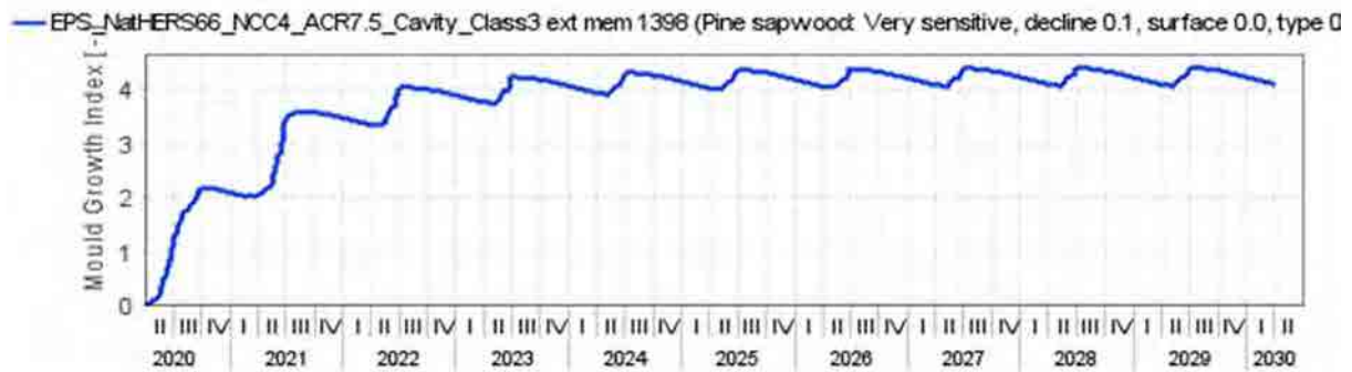
Figure 105: Expanded Polystyrene (EPS) NatHERS CZ 66 - NCC CZ 4 South orientation ACR 7.5, With Cavity – Ext. Memb. Class 3 – 1398 – Mould growth within insulated timber frame
