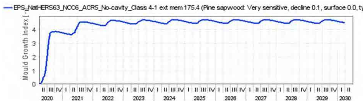
Figure 332: Expanded Polystyrene (EPS) NatHERS CZ 63 - NCC CZ 6 South orientation ACR 5 No Cavity – Ext. Memb. Class 4 – 175.4 – Mould growth within insulated timber frame
