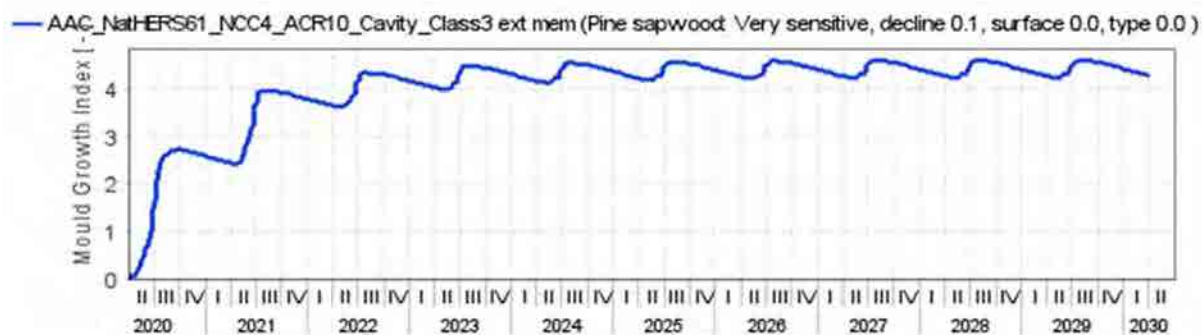
Figure 26: Autoclaved aerated concrete masonry NatHERS CZ 61 - NCC CZ 4 South orientation ACR 10 With Cavity – Ext. Memb. Class 3 – 1398 Mould growth within insulated timber frame
