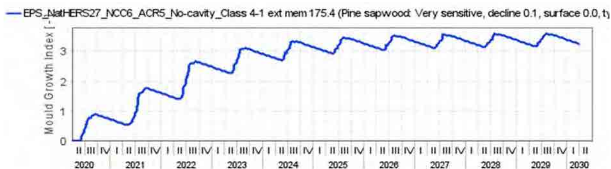
Figure 224: Expanded Polystyrene (EPS) NatHERS CZ 27 - NCC CZ 6 South orientation ACR 5 No Cavity – Ext. Memb. Class 4 – 175.4 – Mould growth within insulated timber frame
