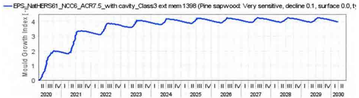
Figure 287: Expanded Polystyrene (EPS) NatHERS CZ 61 - NCC CZ 6 South orientation ACR 7.5, With Cavity – Ext. Memb. Class 3 – 1398 – Mould growth within insulated timber frame
