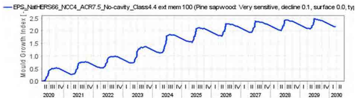
Figure 102 Expanded Polystyrene (EPS) NatHERS CZ 66 - NCC CZ 4 South orientation ACR 7.5 No Cavity – Ext. Memb. Class 4 – 100 – Mould growth within insulated timber frame
