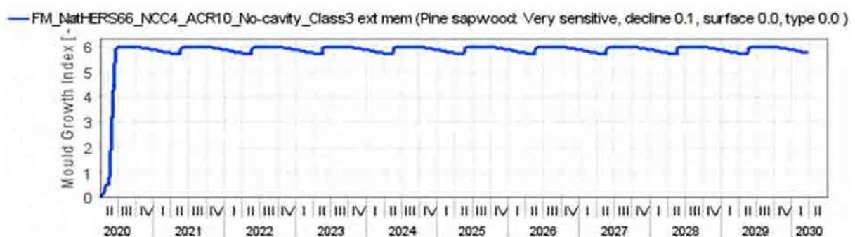
Figure 86: Flat Metal Cladding NatHERS CZ 66 - NCC CZ 4 South orientation ACR 10 No Cavity – Ext. Memb. Class 3 – 1398 – Mould growth within insulated timber frame
