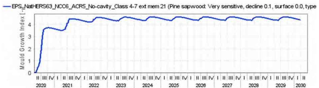
Figure 334: Expanded Polystyrene (EPS) NatHERS CZ 63 - NCC CZ 6 South orientation ACR 5 No Cavity – Ext. Memb. Class 4 – 21 – Mould growth within insulated timber frame
