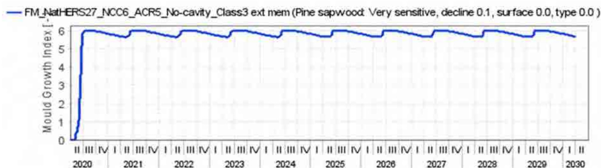
Figure 223: Flat Metal Cladding NatHERS CZ 27 - NCC CZ 6 South orientation ACR 5 No Cavity – Ext. Memb. Class 3 – 1398 – Mould growth within insulated timber frame
