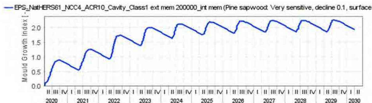
Figure 55: Expanded Polystyrene (EPS) NatHERS CZ 61 - NCC CZ 4 South orientation ACR 10 With Cavity – Ext. Memb. Class 1 – 200000 with Int. Memb. Mould growth within insulated timber frame
