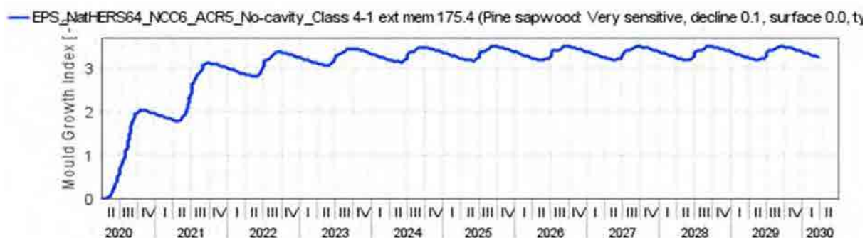
Figure 368: Expanded Polystyrene (EPS) NatHERS CZ 64 - NCC CZ 6 South orientation ACR 5 No Cavity – Ext. Memb. Class 4 – 175.4 – Mould growth within insulated timber frame
