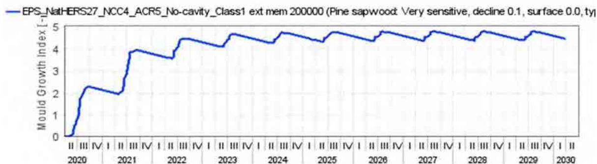
Figure 29: Expanded Polystyrene (EPS) NatHERS CZ 27 - NCC CZ 4 South orientation ACR 5 No Cavity – Ext. Memb. Class 1 – 200000 – Mould growth within insulated timber frame
