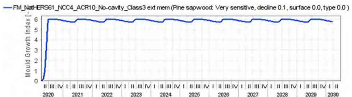
Figure 44: Flat Metal Cladding NatHERS CZ 61 - NCC CZ 4 South orientation ACR 10 No Cavity – Ext. Memb. Class 3 – 1398 – Mould growth within insulated timber frame
