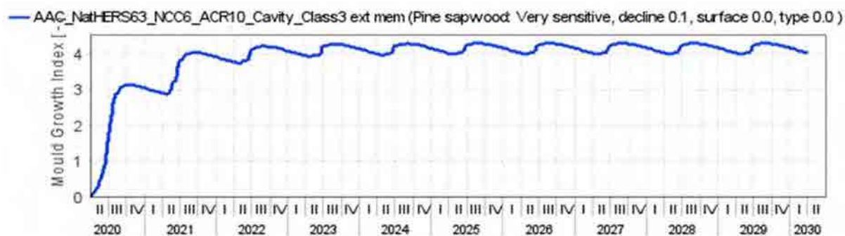
Figure 163: Autoclaved aerated concrete masonry NatHERS CZ 63 - NCC CZ 6 South orientation ACR 10 With Cavity – Ext. Memb. Class 3 – 1398 Mould growth within insulated timber frame
