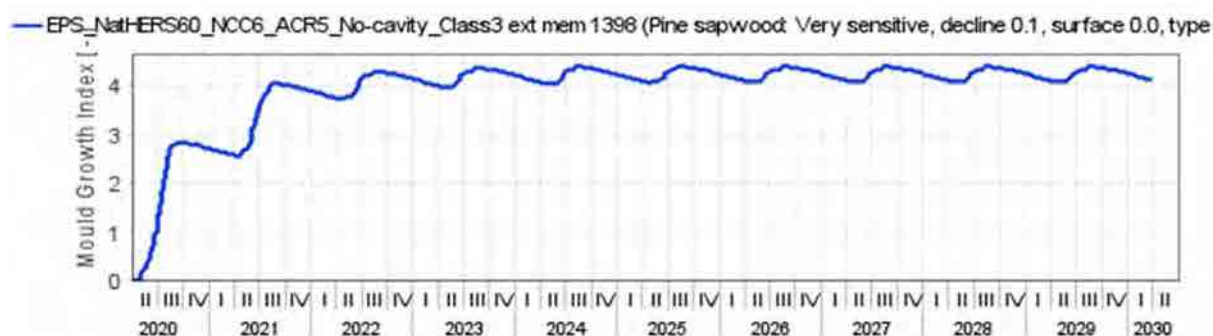
Figure 259: Expanded Polystyrene (EPS) NatHERS CZ 60 - NCC CZ 6 South orientation ACR 5 No Cavity – Ext. Memb. Class 3 – 1398 – Mould growth within insulated timber frame
