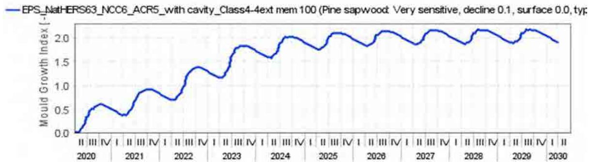
Figure 337 Expanded Polystyrene (EPS) NatHERS CZ 63 - NCC CZ 6 South orientation ACR 5 With Cavity – Ext. Memb. Class 4 – 100 – Mould growth within insulated timber frame
