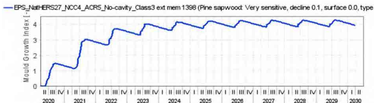
Figure 30: Expanded Polystyrene (EPS) NatHERS CZ 27 - NCC CZ 4 South orientation ACR 5 No Cavity – Ext. Memb. Class 3 – 1398 – Mould growth within insulated timber frame
