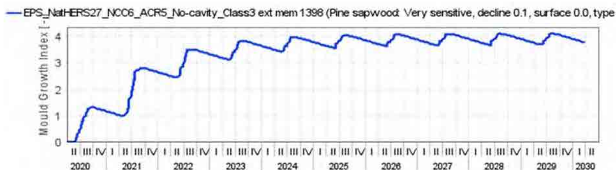
Figure 223: Expanded Polystyrene (EPS) NatHERS CZ 27 - NCC CZ 6 South orientation ACR 5 No Cavity – Ext. Memb. Class 3 – 1398 – Mould growth within insulated timber frame
