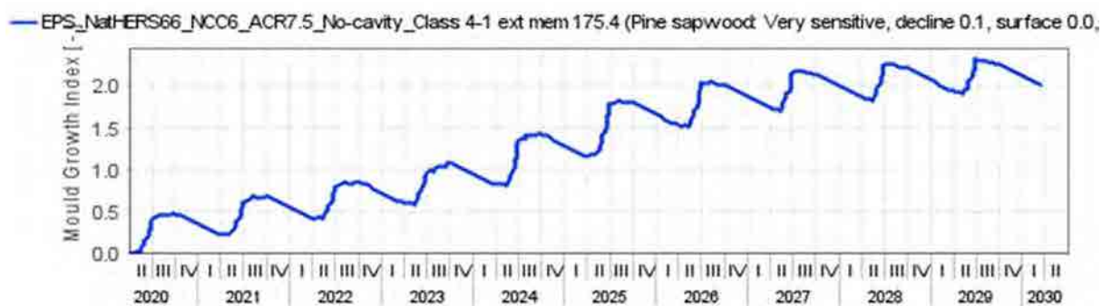
Figure 392: Expanded Polystyrene (EPS) NatHERS CZ 66 - NCC CZ 6 South orientation ACR 7.5, No Cavity – Ext. Memb. Class 4 – 175.4 – Mould growth within insulated timber frame
