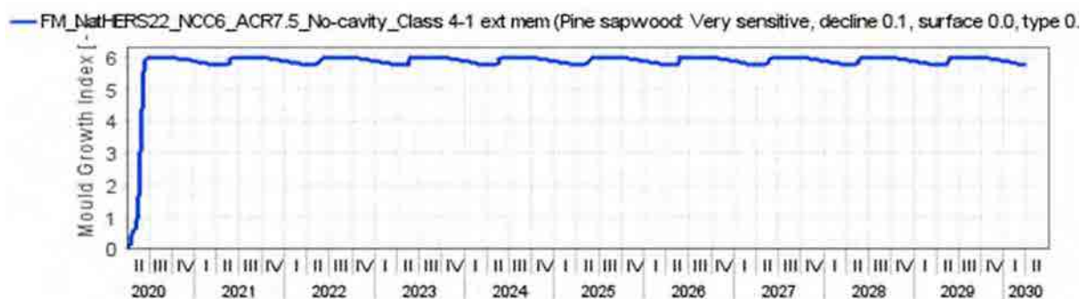
Figure 176: Flat Metal Cladding NatHERS CZ 22 - NCC CZ 6 South orientation ACR 7.5 No Cavity – Ext. Memb. Class 4 – 175.4 – Mould growth within insulated timber frame
