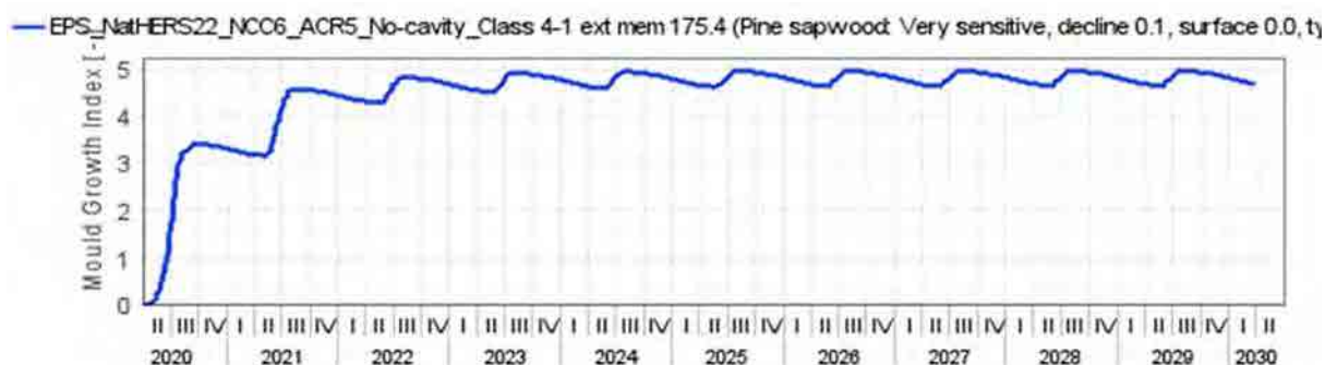
Figure 188: Expanded Polystyrene (EPS) NatHERS CZ 22 - NCC CZ 6 South orientation ACR 5 No Cavity – Ext. Memb. Class 4 – 175.4 – Mould growth within insulated timber frame
