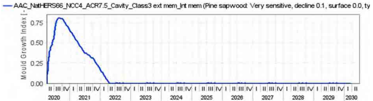
Figure 63 Autoclaved aerated concrete masonry NatHERS CZ 66 - NCC CZ 4 South orientation ACR 7.5 With Cavity – Ext. Memb. Class 4 – 1398 with Int. Memb. Mould growth within insulated timber frame
