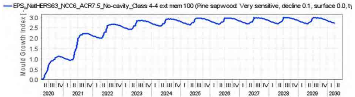
Figure 321 Expanded Polystyrene (EPS) NatHERS CZ 63 - NCC CZ 6 South orientation ACR 7.5 No Cavity – Ext. Memb. Class 4 – 100 – Mould growth within insulated timber frame
