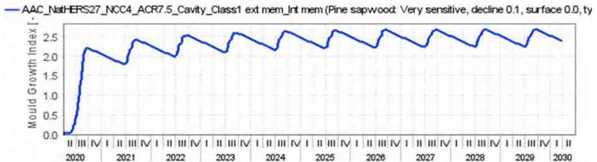
Figure 14 Autoclaved aerated concrete masonry NatHERS CZ 27 - NCC CZ 4 South orientation ACR 7.5 With Cavity – Ext. Memb. Class1 – 200000 with Int. Memb. Mould growth within insulated timber frame
