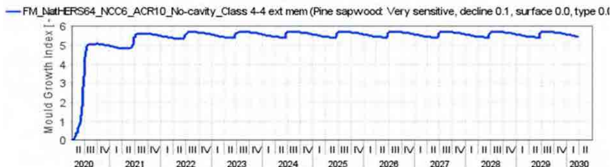
Figure 345 Flat Metal Cladding NatHERS CZ 64 - NCC CZ 6 South orientation ACR 10 No Cavity – Ext. Memb. Class 4 – 100 – Mould growth within insulated timber frame
