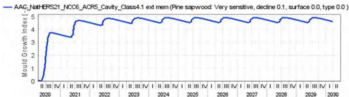
Figure 86: Autoclaved aerated concrete masonry NatHERS CZ 21 - NCC CZ 6 South orientation ACR 5 With Cavity – Ext. Memb. Class 4 – 175.4 Mould growth within insulated timber frame
