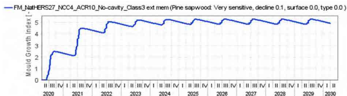
Figure 2: Flat Metal Cladding NatHERS CZ 27 - NCC CZ 4 South orientation ACR 10 No Cavity – Ext. Memb. Class 3 – 1398 – Mould growth within insulated timber frame
