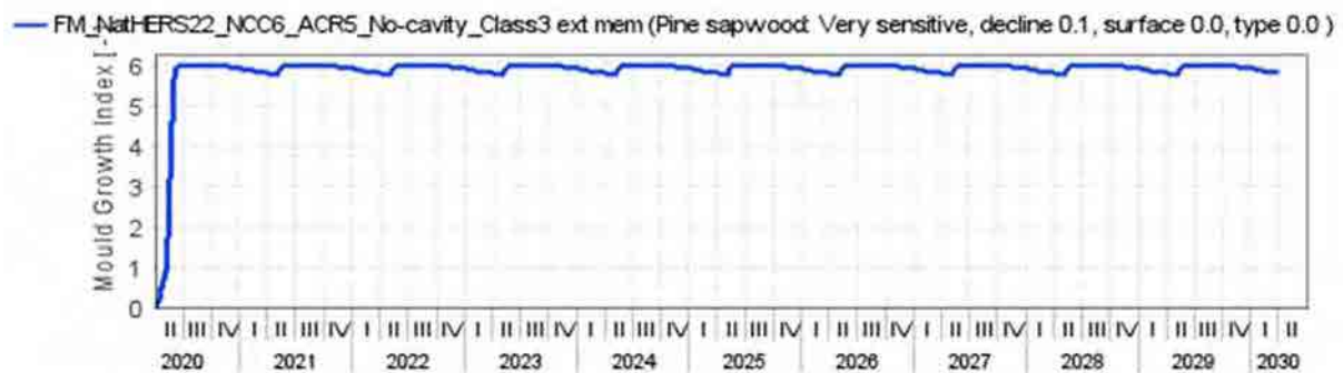
Figure 199: Flat Metal Cladding NatHERS CZ 27 - NCC CZ 6 South orientation ACR 10 No Cavity – Ext. Memb. Class 3 – 1398 – Mould growth within insulated timber frame
