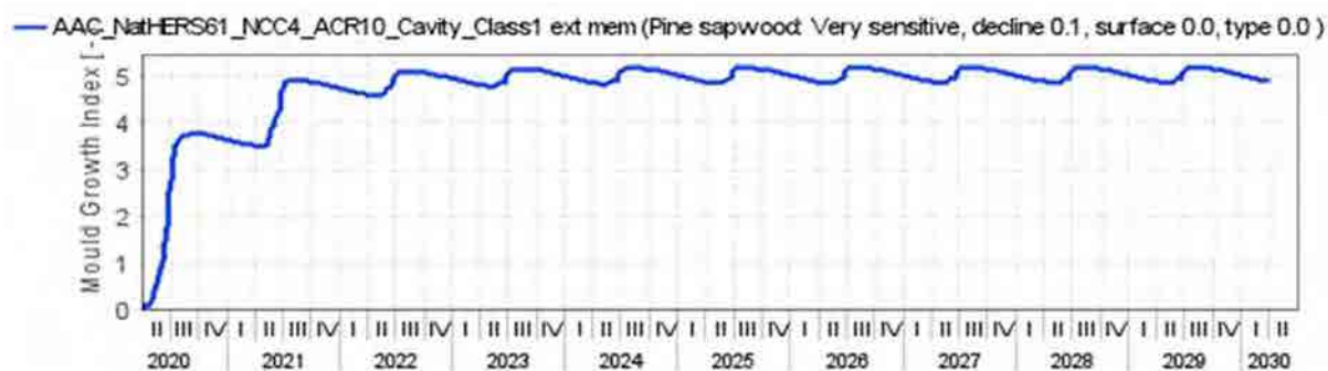
Figure 25: Autoclaved aerated concrete masonry NatHERS CZ 61 - NCC CZ 4 South orientation ACR 10 With Cavity – Ext. Memb. Class 1 – 200000 Mould growth within insulated timber frame
