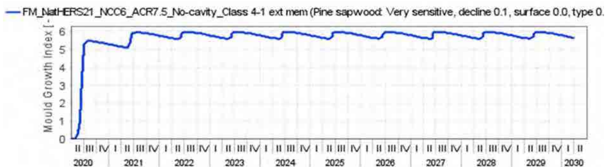
Figure 140: Flat Metal Cladding NatHERS CZ 21 - NCC CZ 6 South orientation ACR 7.5 No Cavity – Ext. Memb. Class 4 – 175.4 – Mould growth within insulated timber frame
