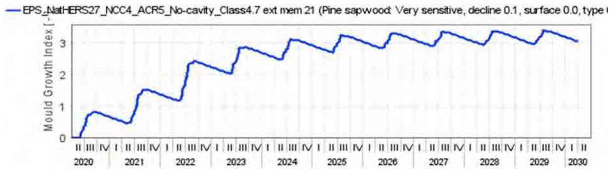
Figure 33: Expanded Polystyrene (EPS) NatHERS CZ 27 - NCC CZ 4 South orientation ACR 5 No Cavity – Ext. Memb. Class 4 – 21 – Mould growth within insulated timber frame
