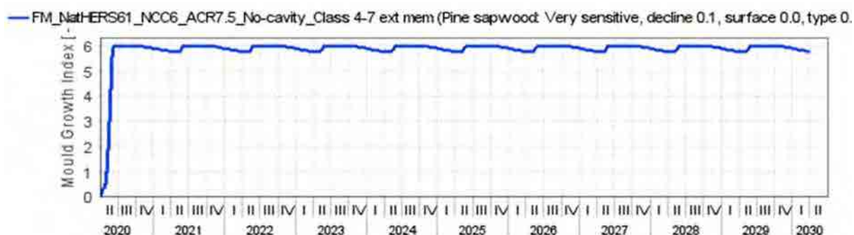
Figure 286: Flat Metal Cladding NatHERS CZ 61 - NCC CZ 6 South orientation ACR 7.5 No Cavity – Ext. Memb. Class 4 – 21 – Mould growth within insulated timber frame
