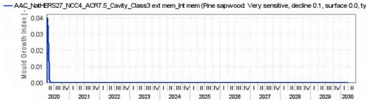
Figure 15 Autoclaved aerated concrete masonry NatHERS CZ 27 - NCC CZ 4 South orientation ACR 7.5 With Cavity – Ext. Memb. Class 4 – 1398 with Int. Memb. Mould growth within insulated timber frame
