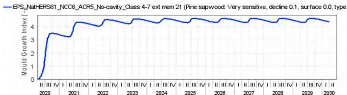
Figure 298: Expanded Polystyrene (EPS) NatHERS CZ 61 - NCC CZ 6 South orientation ACR 5 No Cavity – Ext. Memb. Class 4 – 21 – Mould growth within insulated timber frame
