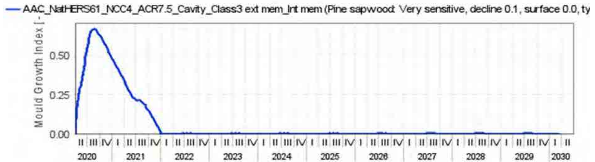
Figure 39 Autoclaved aerated concrete masonry NatHERS CZ 61 - NCC CZ 4 South orientation ACR 7.5 With Cavity – Ext. Memb. Class 4 – 1398 with Int. Memb. Mould growth within insulated timber frame
