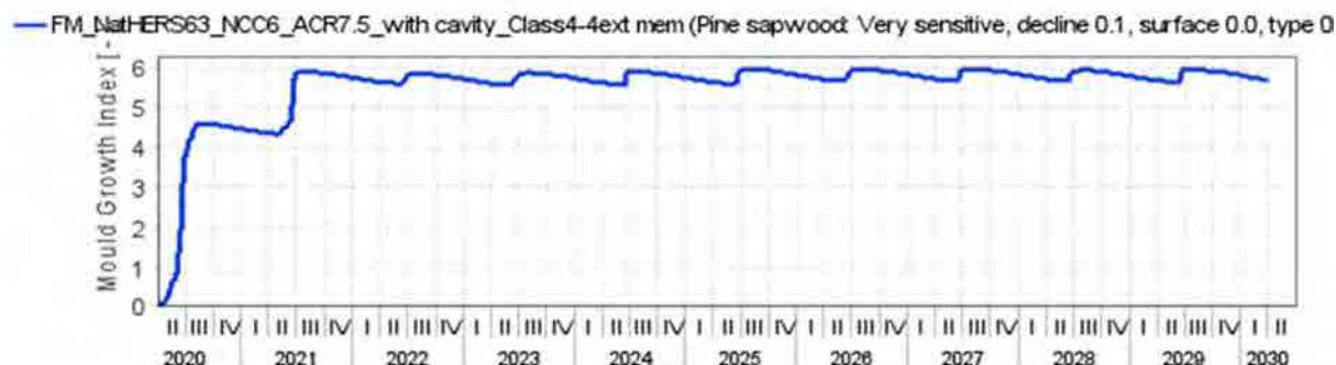
Figure 325 Flat Metal Cladding NatHERS CZ 63 - NCC CZ 6 South orientation ACR 7.5 With Cavity – Ext. Memb. Class 4 – 100 – Mould growth within insulated timber frame
