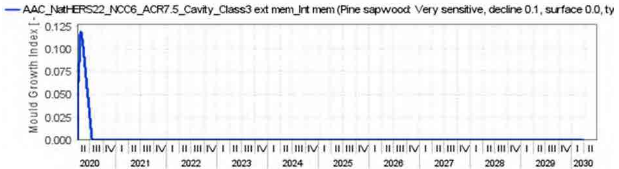
Figure 101 Autoclaved aerated concrete masonry NatHERS CZ 22 - NCC CZ 6 South orientation ACR 7.5 With Cavity – Ext. Memb. Class 4 – 1398 with Int. Memb. Mould growth within insulated timber frame
