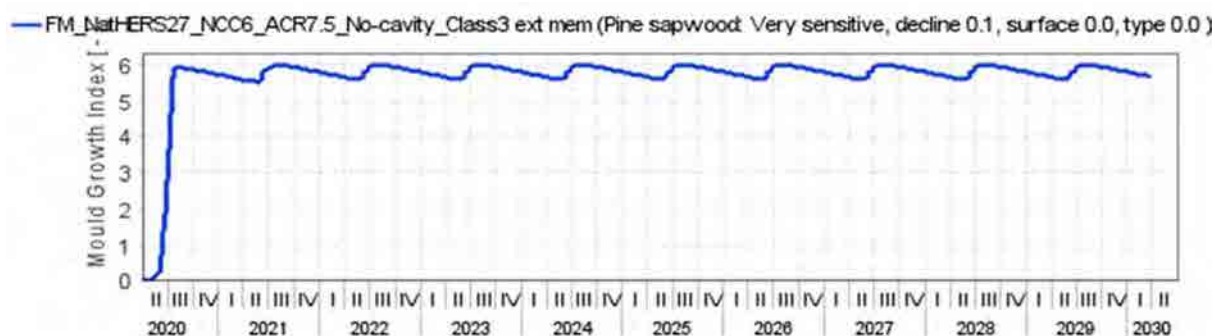
Figure 211: Flat Metal Cladding NatHERS CZ 27 - NCC CZ 6 South orientation ACR 7.5 No Cavity – Ext. Memb. Class 3 – 1398 – Mould growth within insulated timber frame
