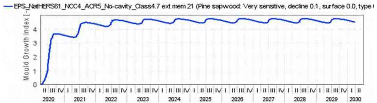
Figure 75: Expanded Polystyrene (EPS) NatHERS CZ 61 - NCC CZ 4 South orientation ACR 5 No Cavity – Ext. Memb. Class 4 – 21 – Mould growth within insulated timber frame
