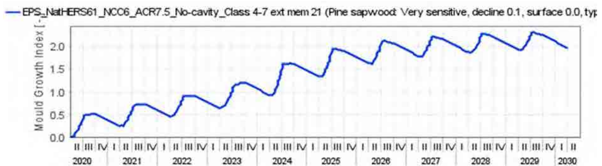
Figure 286: Expanded Polystyrene (EPS) NatHERS CZ 61 - NCC CZ 6 South orientation ACR 7.5 No Cavity – Ext. Memb. Class 4 – 21 – Mould growth within insulated timber frame
