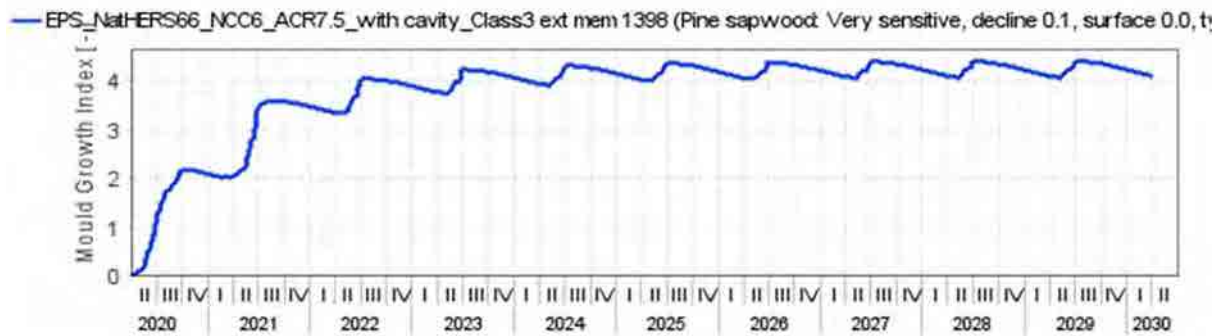
Figure 395: Expanded Polystyrene (EPS) NatHERS CZ 66 - NCC CZ 6 South orientation ACR 7.5, With Cavity – Ext. Memb. Class 3 – 1398 – Mould growth within insulated timber frame
