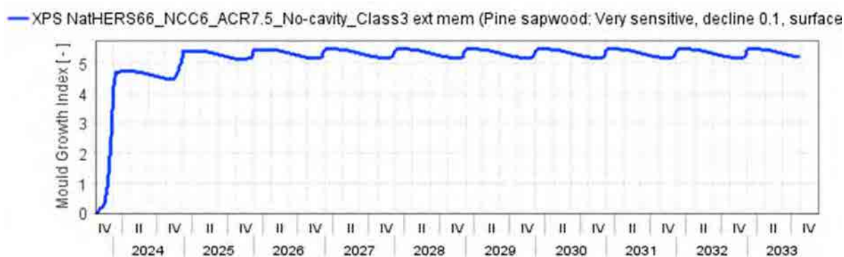
Figure 391: 7 STAR XPS NatHERS CZ 66 - NCC CZ 6 South orientation ACR 7.5, No Cavity – Ext. Memb. Class 4 – 175.4 – Mould growth within insulated timber frame
