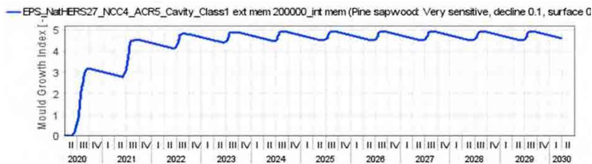
Figure 41: Expanded Polystyrene (EPS) NatHERS CZ 27 - NCC CZ 4 South orientation ACR 5 With Cavity – Ext. Memb. Class 1 – 200000 with Int. Memb. Mould growth within insulated timber frame
