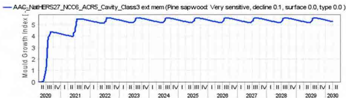
Figure 121: Autoclaved aerated concrete masonry NatHERS CZ 27 - NCC CZ 6 South orientation ACR 5 With Cavity – Ext. Memb. Class 3 – 1398 Mould growth within insulated timber frame
