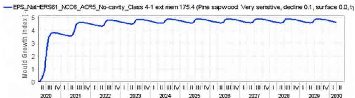
Figure 296: Expanded Polystyrene (EPS) NatHERS CZ 61 - NCC CZ 6 South orientation ACR 5 No Cavity – Ext. Memb. Class 4 – 175.4 – Mould growth within insulated timber frame
