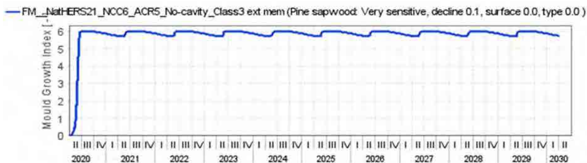
Figure 151: Flat Metal Cladding NatHERS CZ 21 - NCC CZ 6 South orientation ACR 5 No Cavity – Ext. Memb. Class 3 – 1398 – Mould growth within insulated timber frame
