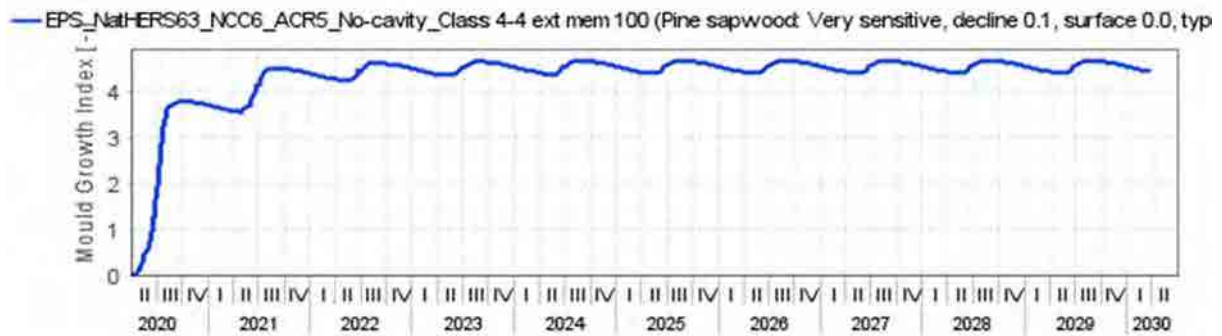
Figure 333 Expanded Polystyrene (EPS) NatHERS CZ 63 - NCC CZ 6 South orientation ACR 5 No Cavity – Ext. Memb. Class 4 – 100 – Mould growth within insulated timber frame
