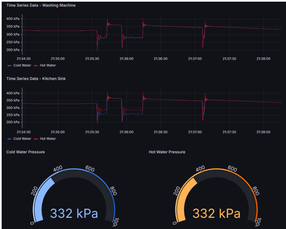
Figure 3 - Example of dashboard for study households to view live pressure data.
