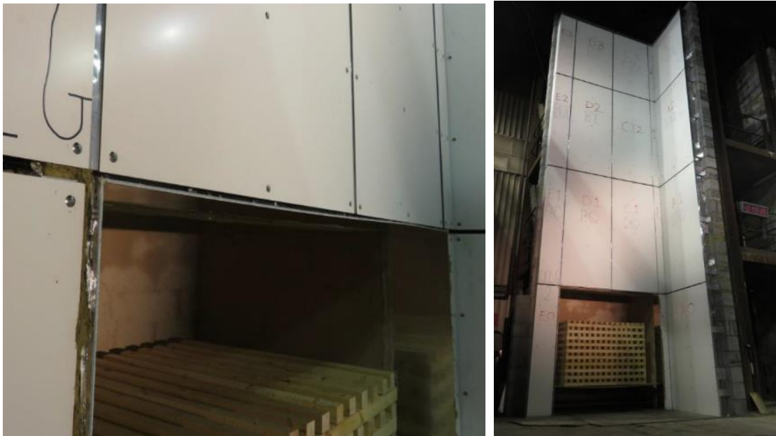
Figure 15. Left – Aluminium window pod, combustion chamber and ACP joints and fixing detail. Right – complete façade system prior to test (all photos taken from BRE Test report
