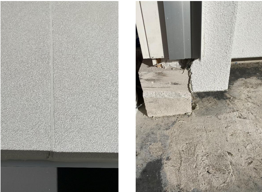
Figure 5. Vertical construction joint (left) and edge of combustion chamber (right) showing simulated timber window reveal and Hebel block simulating slab edge) during CSIRO inspection of completed construction at Warringtonfire.
