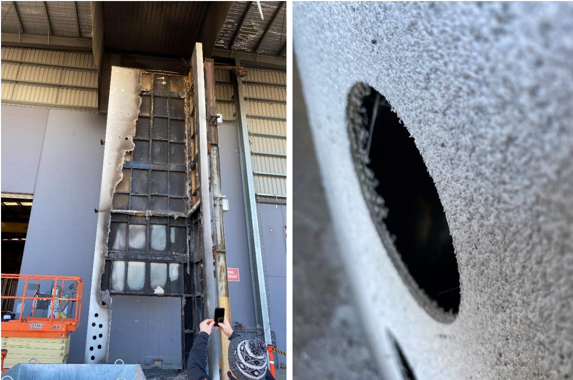
Figure 13. Post-test wall system showing render thickness hole saw samples. Right photo shows close up hole saw sample on left side of combustion chamber with EPS behind completely melted/burnt away.
