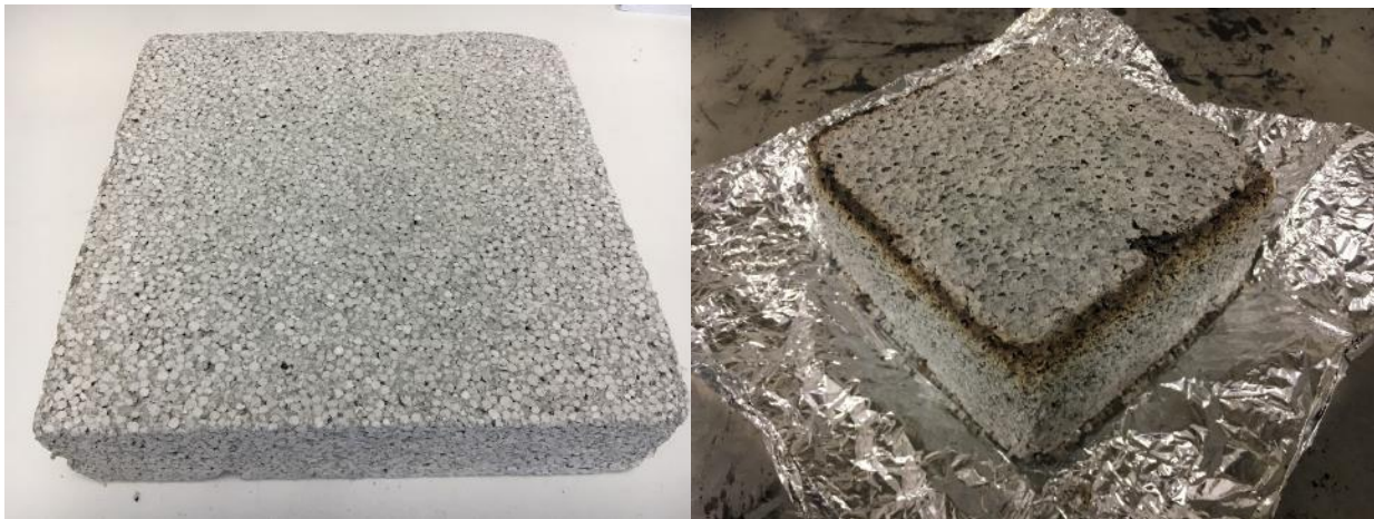
Figure 26. Compolcrete prior to cone calorimeter test (left) and after cone calorimeter test (right) – All photos by CSIRO
