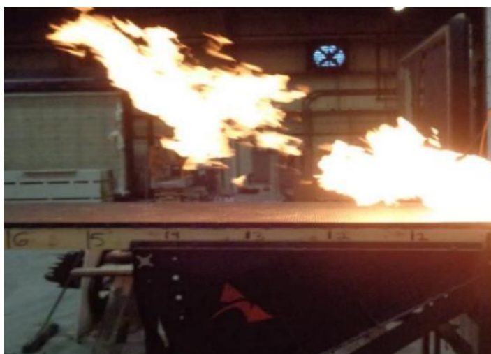
Figure 73. ASTM E-108 Spread of flame test
