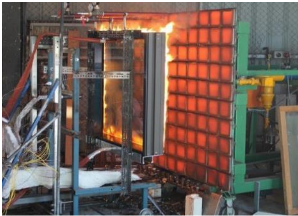
Figure 75. CSIRO pilot scale AS 1530.8.1 test (left), BAL radiant heat test profiles (right)
