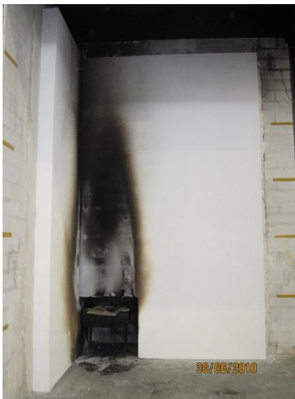
Figure 81. DIN 4102-20 (Draft) test rig (From BRE Global [159] )
