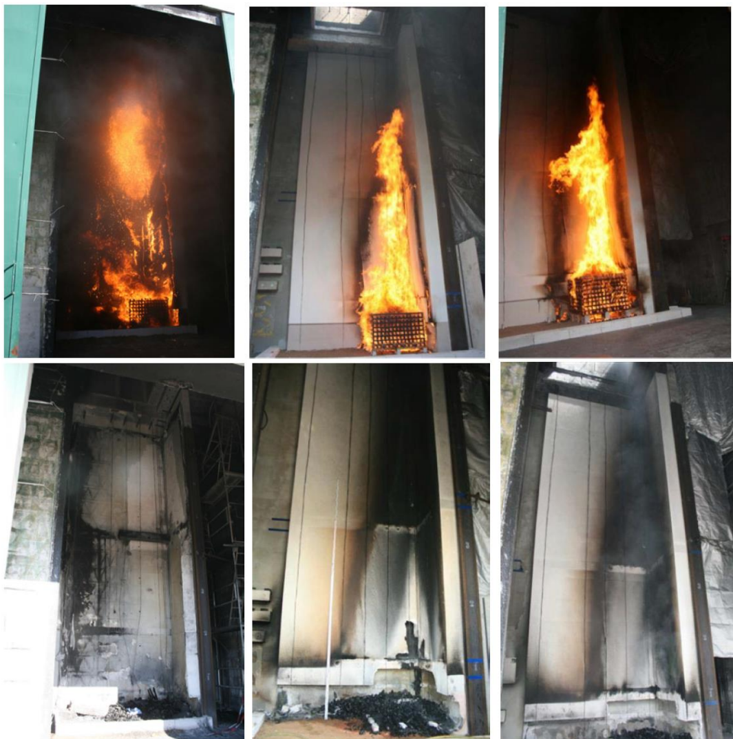
Figure 89. Test 1 at 15 min and post-test (left); Test 2 and 3 at 18 min and post-test (middle and right) [167]
